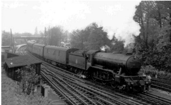
Class K3 2-6-0 no.61843 rounds the curve at Rickmansworth with an up passenger. photo : © L.V.Reason
